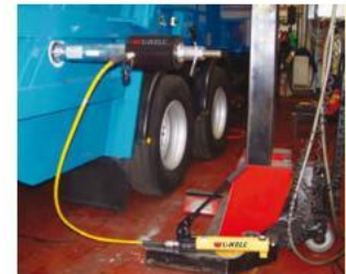
一個RACH-306油缸由P-392手動泵提供動力，將廢品回收車車架上已被腐蝕的銷子拔出。 An RACH-306 powered by a P-392 hand pump used to extract corroded carriage pins of refuse collection vehicles.
